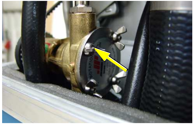
Fig. B.7.3-3: wing screw raw water pump
