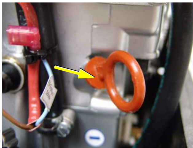
Fig. A.3.8-2: Engine oil dipstick
