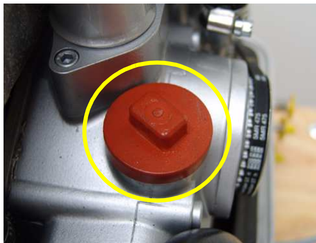
Fig. A.3.8-1: Engine oil filler neck
