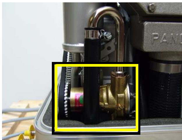
Fig. B.7.3-2: Raw water pump
