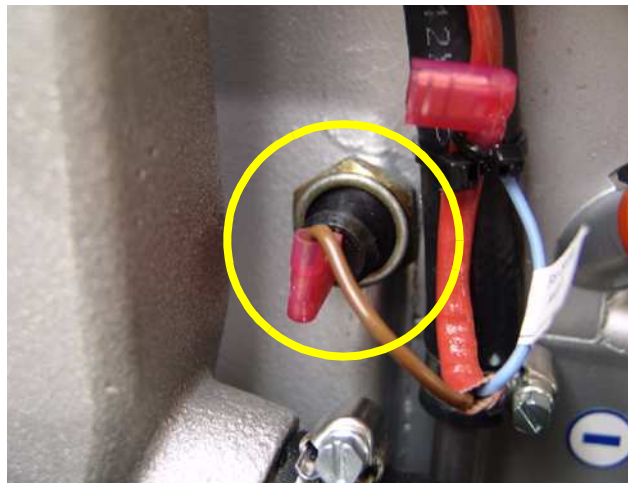
Fig. A.3.7-4: Oil pressure switch
