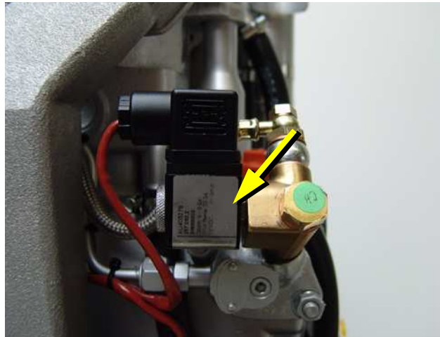
Fig. A.3.4-3: Fuel solenoid valve
