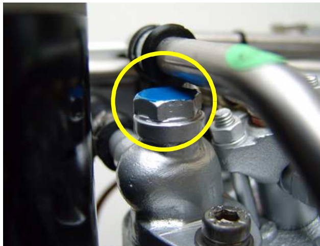
Fig. A.3.3-10: Ventilation screw cylinder head
