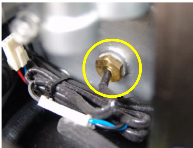
Fig. A.61: Oil sensor at oil sump
